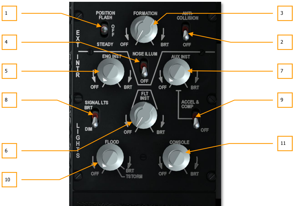
Figure 126. Light Control Panel
