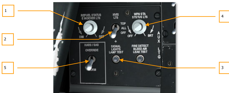
Figure 116. Auxiliary Lighting Control Panel
