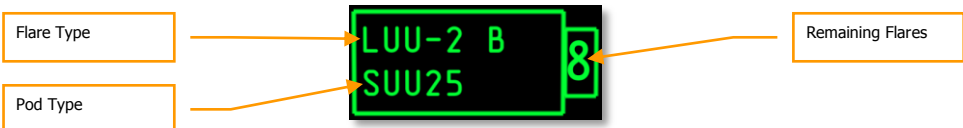
Figure 438. Illumination Flare Station Box
