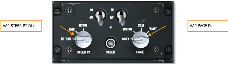
Figure 344. Auxiliary Avionics Panel (AAP)
