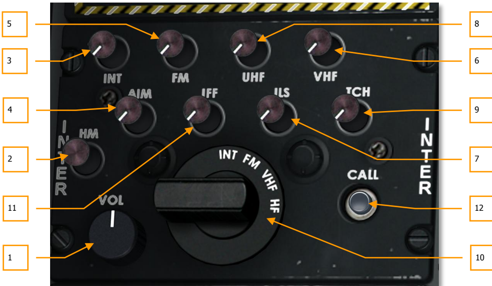
Figure 120. Intercom Control Panel
