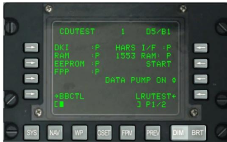
Figure 176. System / CDU Test Sub-Page 1
