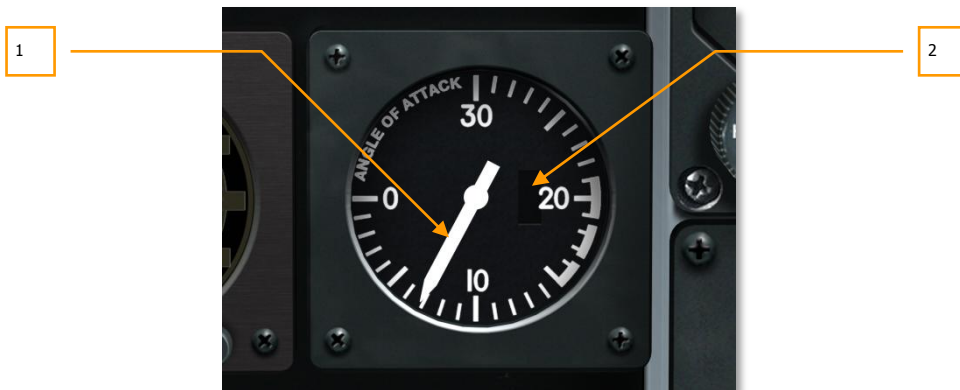
Figure 77. Angle of Attack Indicator
