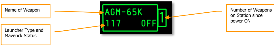
Figure 464. Maverick Station Box Loading, Power Off
