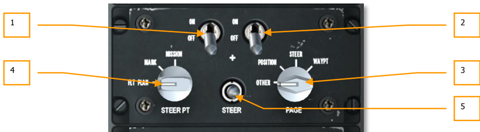
Figure 131. Auxiliary Avionics Panel (AAP)
