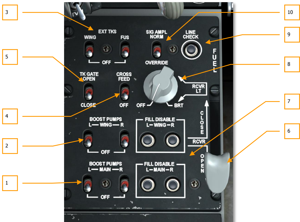
Figure 107. Fuel System Control Panel
