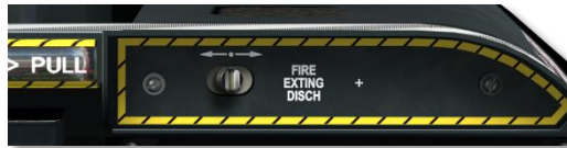
Figure 93. Fire Extinguisher Discharge
