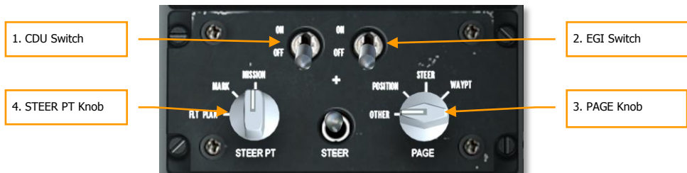
Figure 307. Auxiliary Avionics Panel
