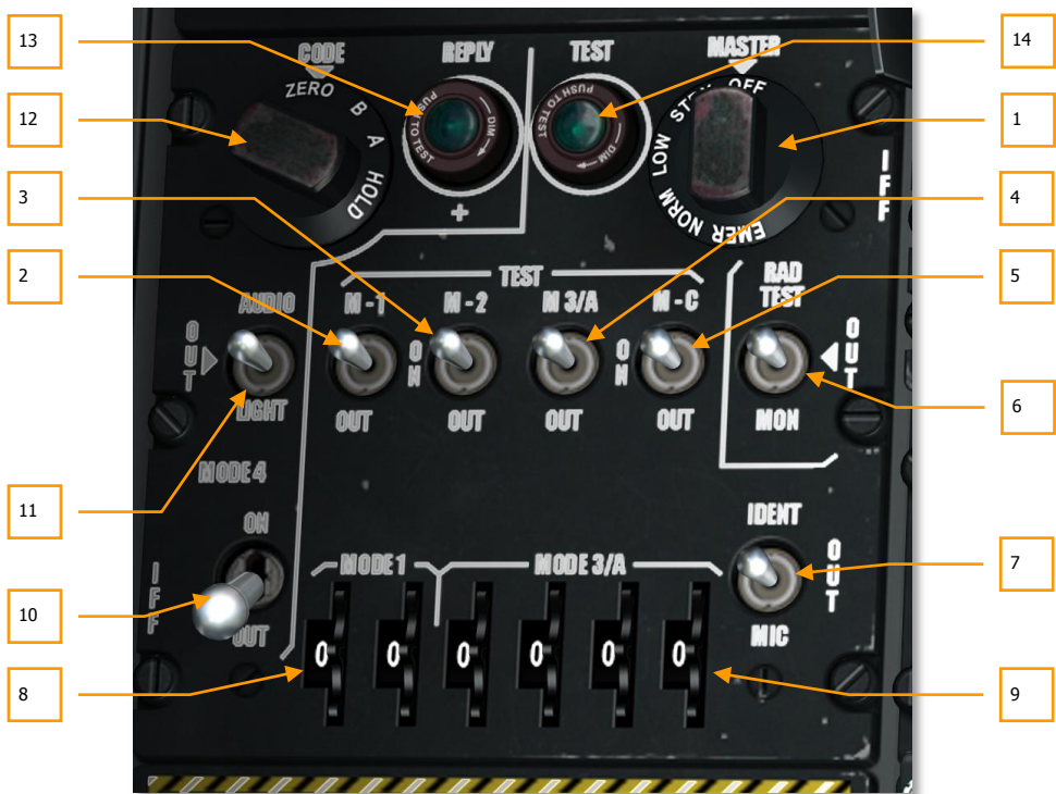
Figure 118. IFF/SIF Control Panel
