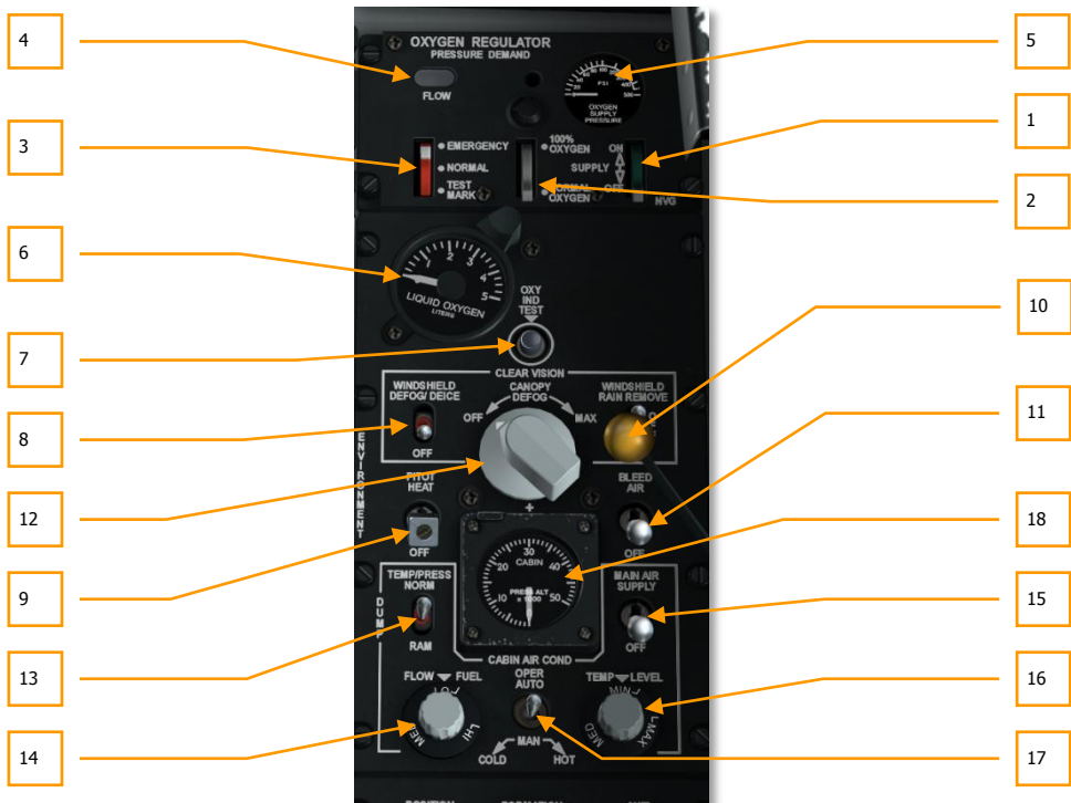
Figure 125. Environment System Panel
