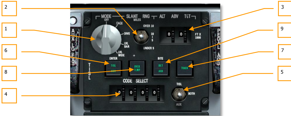
Figure 91. TISL Control Panel
