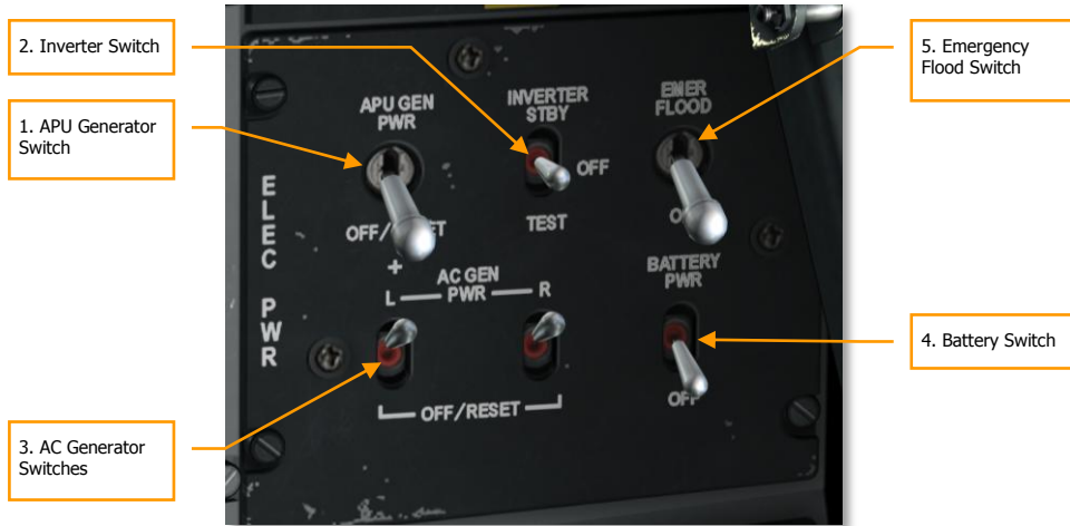
Figure 304. Electrical Power Control Panel
