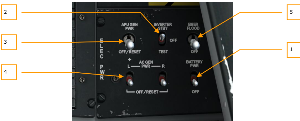
Figure 124. Electrical Power Panel
