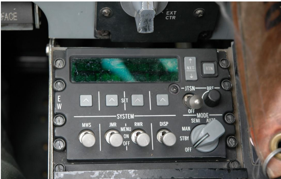
Figure 39. Countermeasure Signal Processor (CMSP) Panel
