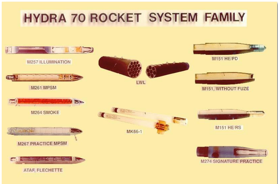
Figure 45. 2.75 inch FFAR Warhead Types
