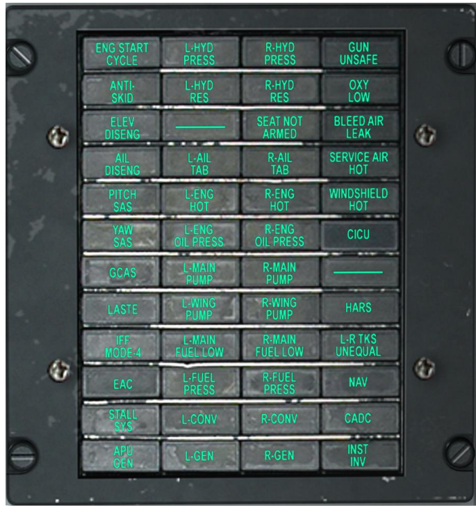
Figure 127. Caution Light Panel
