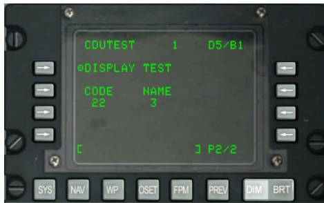
Figure 178. System / CDU Test Sub-Page 2
