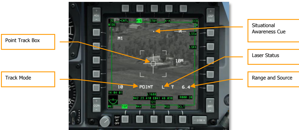
Figure 447. TGP A-G in Point Track
