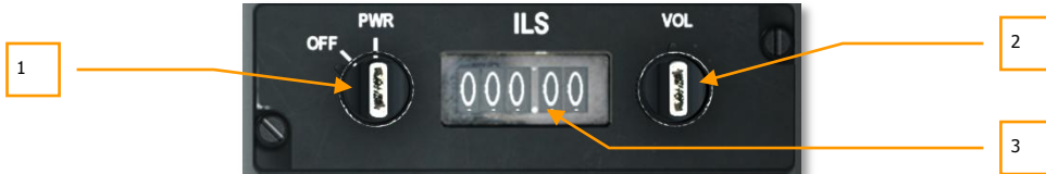
Figure 129. ILS Control Panel
