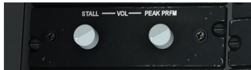
Figure 121. Stall Warning Control Panel
