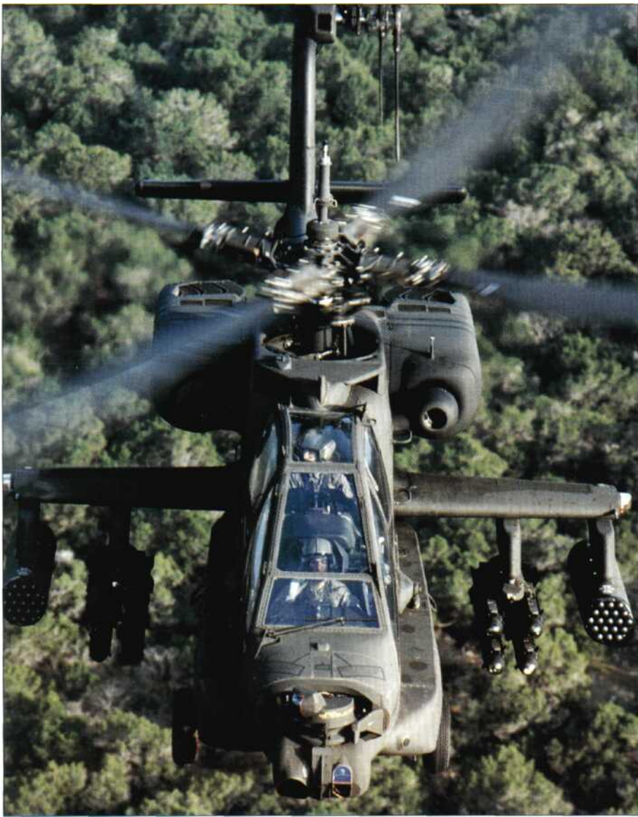
Above: TADS that have been upgraded to OI (optically improved) configuration - that is, most in service - have been modified with a series of optical filters to protect the CPG from laser energy. They will also protect the FUR from video 'bloom' caused by lasers. Four filter settings are available: normal (clear, no protection), S (Short, provides protection against short-wavelength lasers), L (Long, protects against long-wavelength lasers) and MAX (combined L and S filters). The DVO system has filters applied to fixed optics which are thus always in place.
