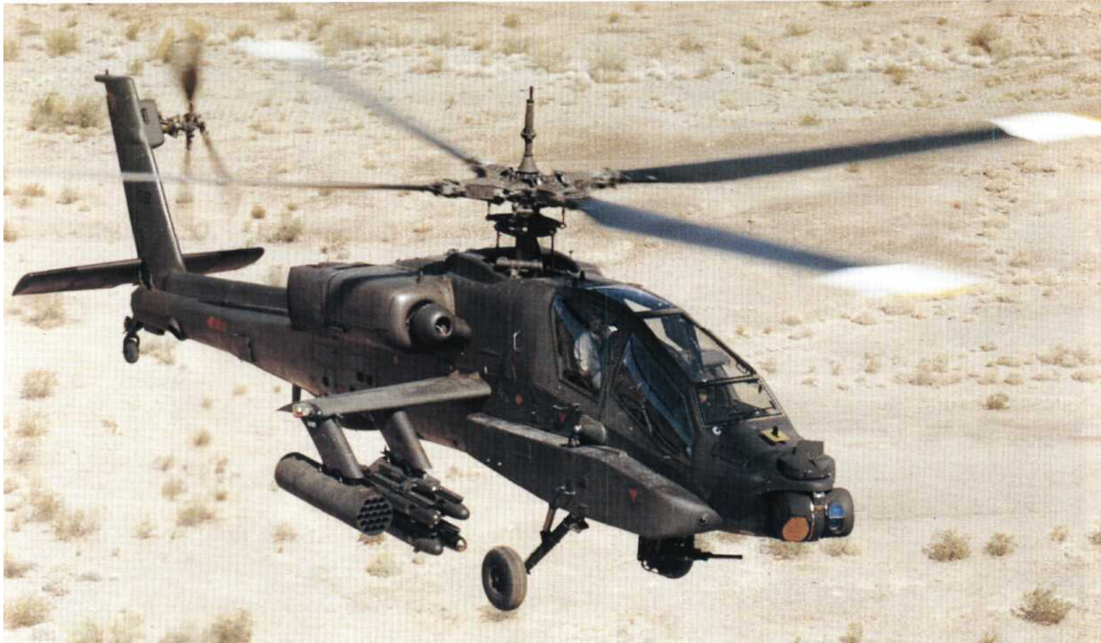
Above: Phase II testing revealed problems with the AH-64's rotor tips. As a result, the blade tips were swept back, leading to a reduction in compression loads and overall noise signature.
