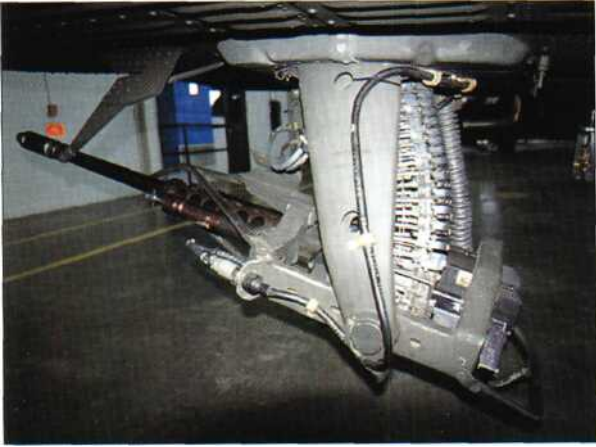
Left and above: The M230E1 30-mm Chain Gun* has a void space above it, to fold into in the event of a crash, protecting the crew. The Chain Gun's 'chain' can be seen above, at the point where it interfaces with the ammunition flatpack. The chain carries rounds to the right to feed the gun
