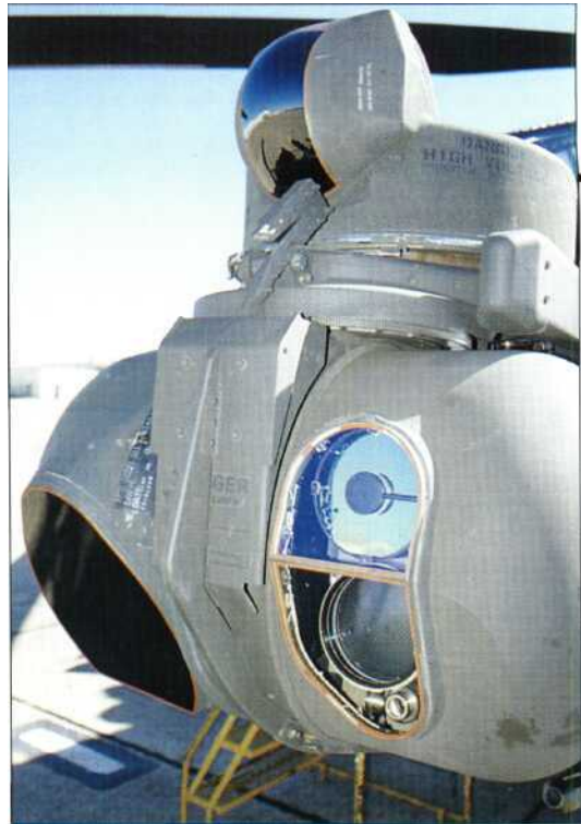
Above: Visible above the TADS optical and laser turret (right) is the LRU-28 transmitting antenna for the Apache's ALQ-136 radar jammer. The Apache's laser - the lower-most of the three components in the turret - is a neodymium-yttrium aluminium garnet (Nd-YAG) laser. The glass panels of the TADS turrets are heated to protect against icing. Note the wire deflector between the turrets and the cutter above them, in front of the PNVs.
