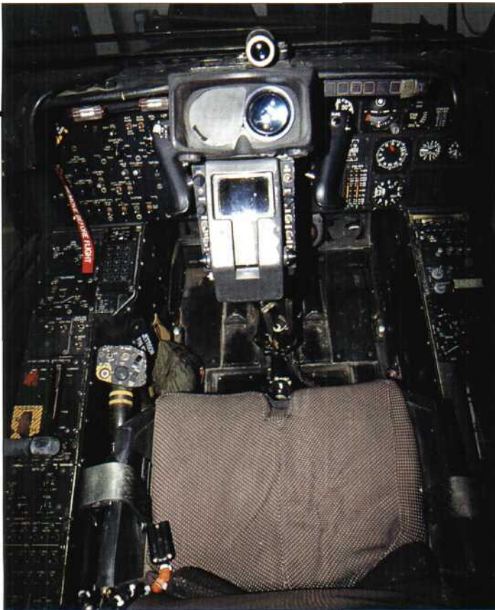
Left: The front (CPG's) cockpit of the AH-64A is dominated by the ORT and its 'T-bar' handgrip. On the front console the CPG has a fire control panel (left) and a set of basic flight instruments (right). On the port side-console (from front to back) can be seen the Hell fire missile control panel, data entry keyboard, anti-icing controls, power lever quadrant, fuel control panel, interior lighting controls and circuit breakers. The starboard side-panel contains the communications system control panel, AN/ARC-186 radio controls, Doppler control panel and a blank area (with provision for KY-58 secure voice control) used for map storage. The pilot and CPG have identical collective controls, but slightly different cyclic grips. The CPG cyclic (centre stick) is folded to the floor in this photograph.
