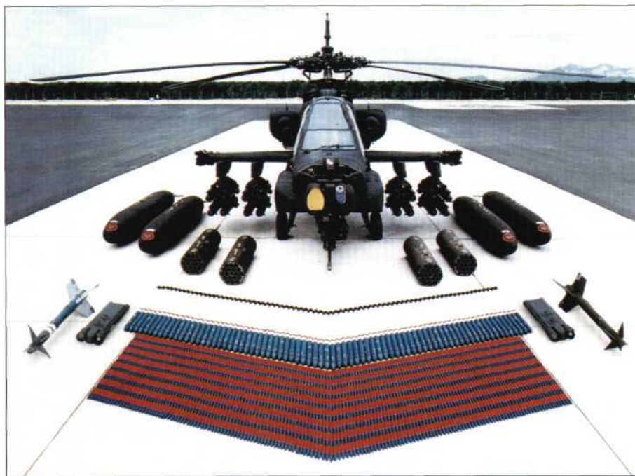
Above: This array of Apache weapons includes Sidewinder and Sidarm missiles (far left, far right), twin Mistral AAMs (foreground), 1,200 rounds of 30-mm shells, 76 2.75-in rockets, 16 Hellfires and wingtip-mounted Stinger AAMs.
