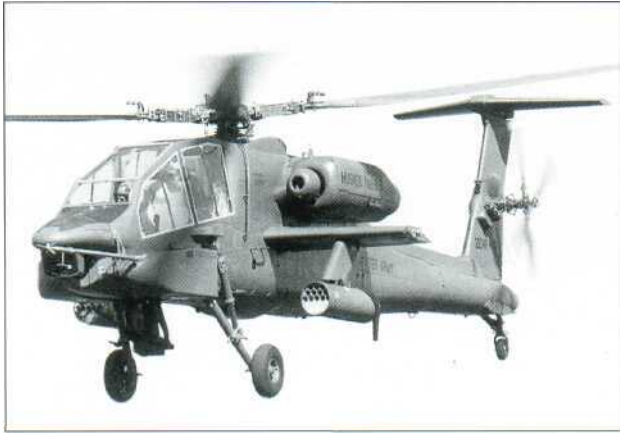
Above: AV-02 (73-22248) was the first YAH-64 to fly. The first to be built (AV-01/73-22247) served its whole life as the GTV (Ground Test Vehicle). AV-02 is seen here soon after its first flight with the original T-tail configuration and mid-set rotor. Several tailplane configurations were tested, including reversing the 'arrowhead' tailplane and adding end-plate fins.
