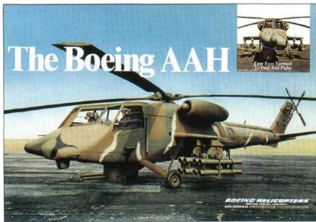
Right: Boeing's AAH entrant featured a novel side-by-side, yet staggered, cockpit arrangement offering "four eyes forward to find and fight," as the brochure put it. Ironically, Boeing is now at the helm of the AH-64 Apache.
