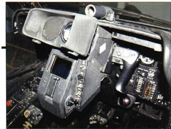
Above: The ORT (Optical Relay Tube) is the primary station where the CPG can monitor TADS/PNVIS imagery, then select, designate and shoot targets. Its bulky construction is also the greatest threat to the CPG's well-being in the event of a crash. The hooded monochrome display at the top can be used head-down, while the screen below allows the CPG to remain 'head-up'. Beneath the open screen are video-source (TADS or PNVIS) and filter selection switches. Flanking the open screen are gain, brightness, grey-scale and FoV adjustment switches. On the left-hand grip can be found the sensor select switch (FLIR, DVO, DTV), weapons action switch (gun, rocket, missile), weapons trigger, primary FoV (wide, medium, narrow, zoom) controls and image autotracking controls. On the right side of the 'T-bar' grip can be found the laser spot tracker controls, manual turret slew controls, FLIR polarity switch (black/white), video recording switch, main laser trigger and boresighting controls.
