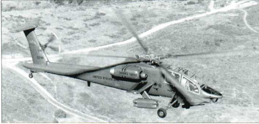
Above: AV-02 (73-22248) was the first YAH-64 to fly. The first to be built (AV-01/73-22247) served its whole life as the GTV (Ground Test Vehicle). AV-02 is seen here soon after its first flight with the original T-tail configuration and mid-set rotor. Several tailplane configurations were tested, including reversing the 'arrowhead' tailplane and adding end-plate fins.
