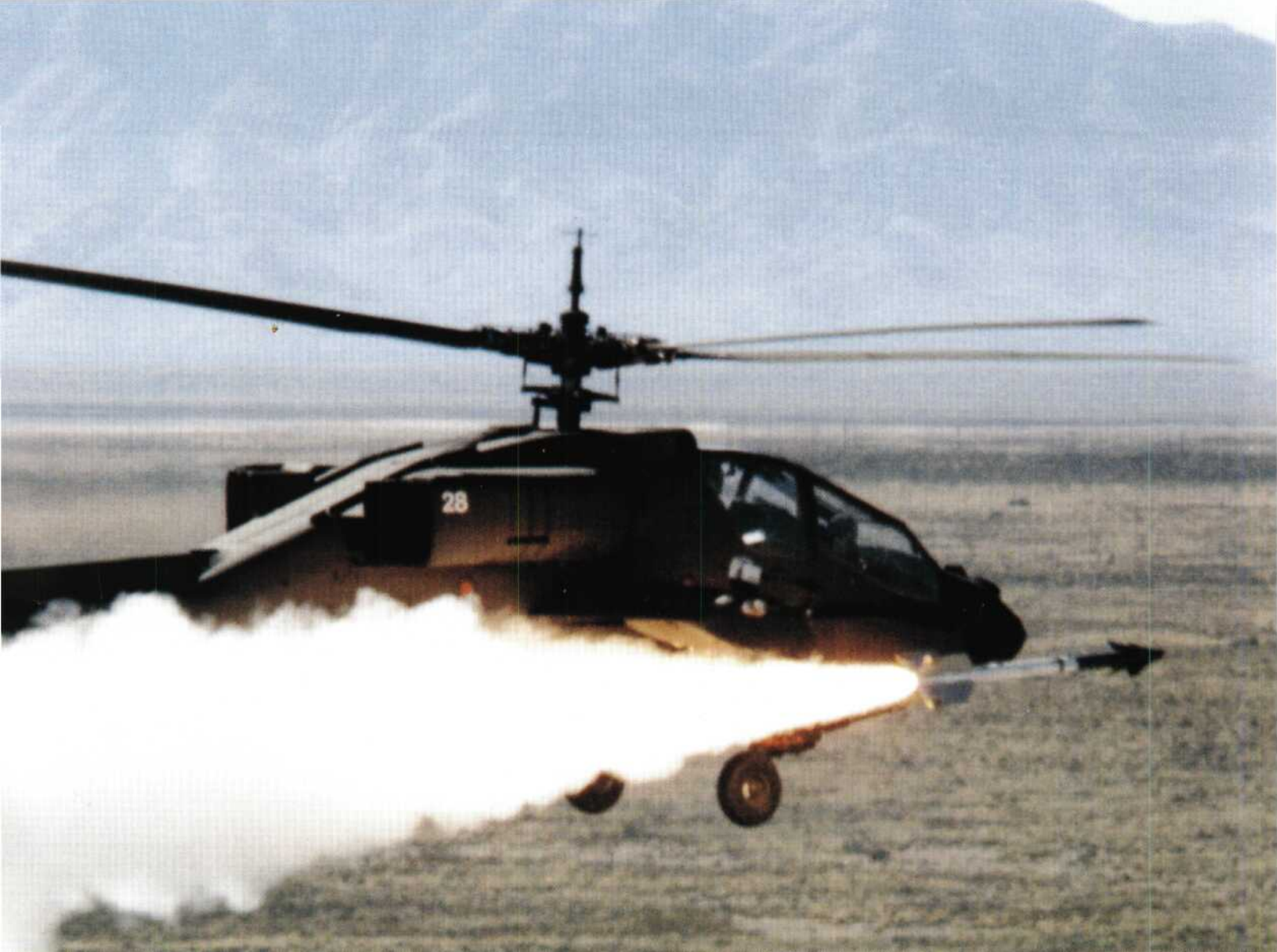
Above: The first launch of a Sidewinder (AIM-9M) was made by an Apache at the White Sands missile range, New Mexico, in November 1987. Several factors led to the adoption of the Stinger missile in favour of the Sidewinder, but one of the most significant of these was the Sidewinder's dramatic launch signature.
