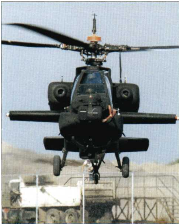
Above: This Ft Hood-based AH-64A (one of the FY84 production batch) is seen in full 'war fit' with Hydra 70 rocket pods, eight Hellfires and M130 chaff dispenser. The pre-production AH-64's had the M130 dispenser attachment point further forward on the tailboom.
