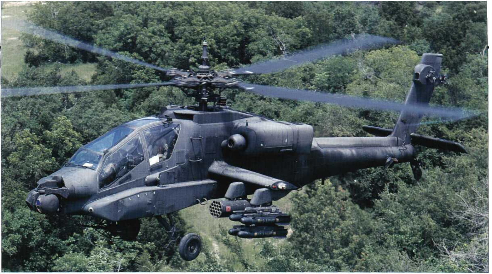
Above: This Ft Hood-based AH-64A (one of the FY84 production batch) is seen in full 'war fit' with Hydra 70 rocket pods, eight Hellfires and M130 chaff dispenser. The pre-production AH-64's had the M130 dispenser attachment point further forward on the tailboom.
