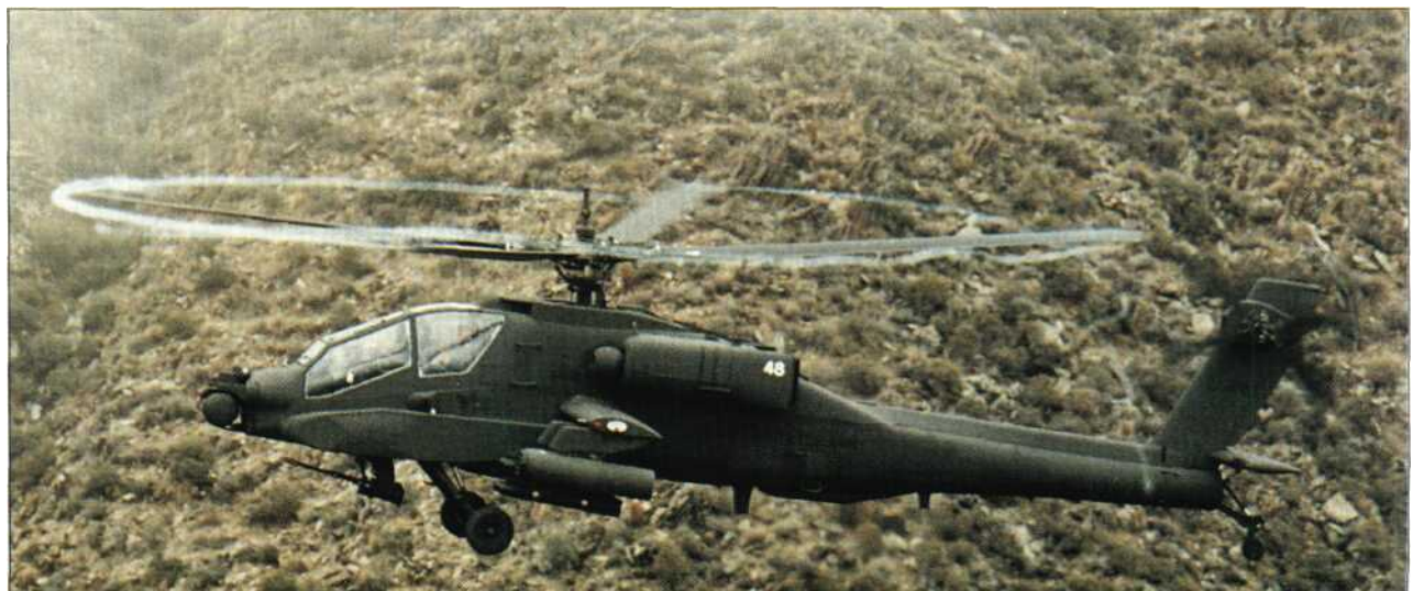
Right: The Apache's fixed rotor mast allows the transmission and gear box to be removed without interfering with the main rotors. The rotor mast is fixed to the fuselage at eight points and, as the rotor drive shaft runs through it, no flight loads are imposed upon the drive shaft itself. This greatly aids the Apache's agility.
