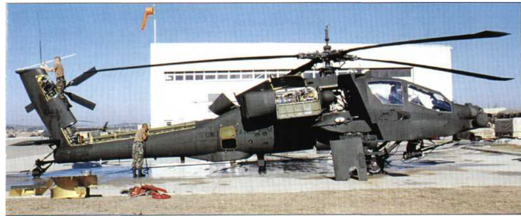
Above: At regular intervals (approximately every 45 days) Apaches are thoroughly washed down. Accumulated dust and dirt can affect the Apache's overall weight by as much as 100 lb (45 kg) if not kept under control. Note how the tailplane can be used as a maintenance platform. The same is true of the engine cowlings.
