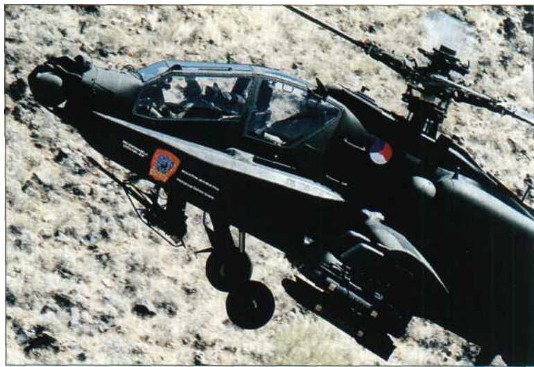
The Dutch Apaches will be AH-64Ds, but without the Longbow radar. This is one of the AH-64D prototypes, wearing a Dutch roundel.
