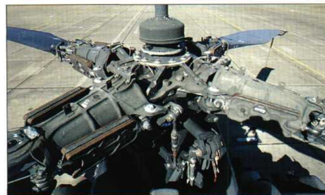
Above: The Apache's rotor head is fully articulated, allowing the blades to 'hunt' (lead or lag) individually. The flexible elastomeric bearings, which regulate this effect, are the large rectangular blocks seen at the end of each blade.
