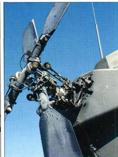
Above: The Apache's rotor blades are each attached to a delta-hinged hub. The whip FM/AM antenna above the fin is not found on all AH-64As. Two AN/APR-39 RWR antennas are located to the rear of the fin cap.
