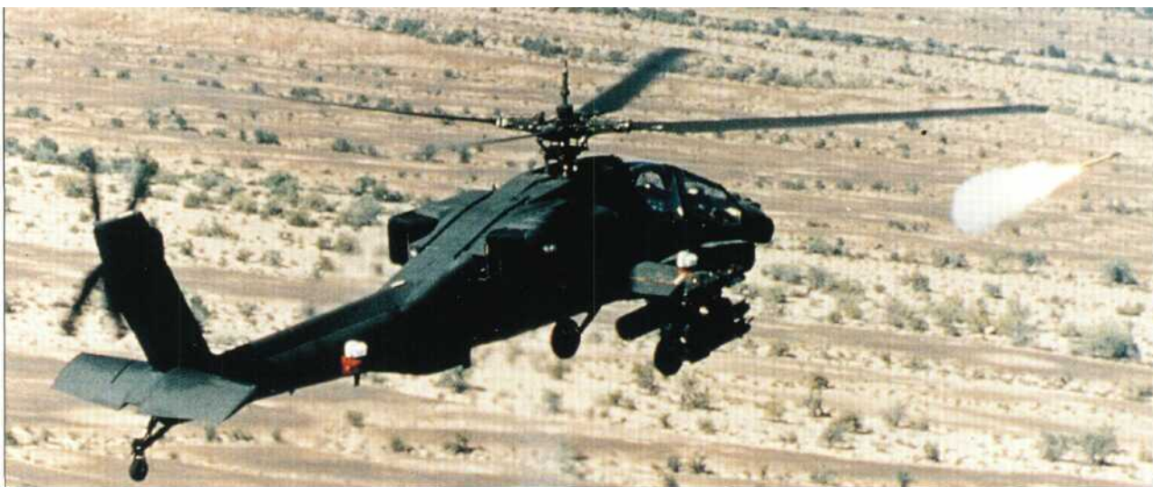
Above: The first launch of a Sidewinder (AIM-9M) was made by an Apache at the White Sands missile range, New Mexico, in November 1987. Several factors led to the adoption of the Stinger missile in favour of the Sidewinder, but one of the most significant of these was the Sidewinder's dramatic launch signature.
