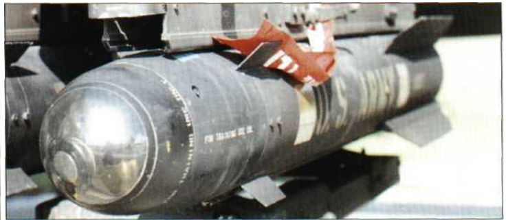
Above and left: All AGM-114 Hellfires are painted black, with olive drab markings. Yellow (3 x 3-in) square markings on the front of the missile denote an HE warhead. Brown squares to the rear signify a solid propellant motor. Inert handling training rounds are designated M34; training rounds with functional seeker heads (above) are M36s.
