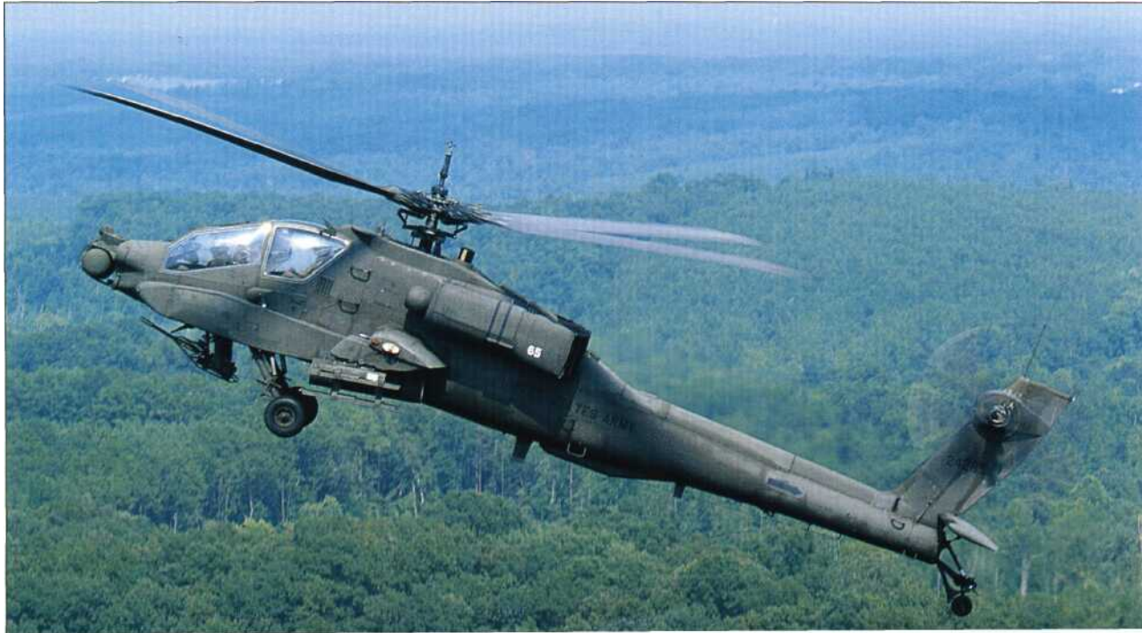
The Apache is fitted with the RT-1296/APX-100(V)1 and RT-1557/APX-100(V) IFF system. APX-100 operates on Modes 1, 2, 3/A, 3/Cand4, transmitting specially coded identification of position or emergency signals as required. Each mode offers progressively more code combinations and ease of use. Mode 4 is the classified operational mode for security identification. IFF antennas are installed on top of the fuselage aft of the canopy, and under the fuselage as an integral part of the UHF-AM antenna. Some Apaches have an IFF antenna located on the work platform forward of the main rotor mast and aft of the tailboom jack pad. IFF transmission from the upper antenna can cause the PNVS to malfunction and slew to the centreline before returning to the pilot's LoS. If this occurs, the transponder must be disengaged or rerouted to the lower antenna.
