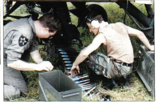
Above: 30-mm rounds are loaded using the motorised uploader/downloader which propels shells up a flex chute, along the port side of the fuselage and into the flatpack or 'ammo can'.
