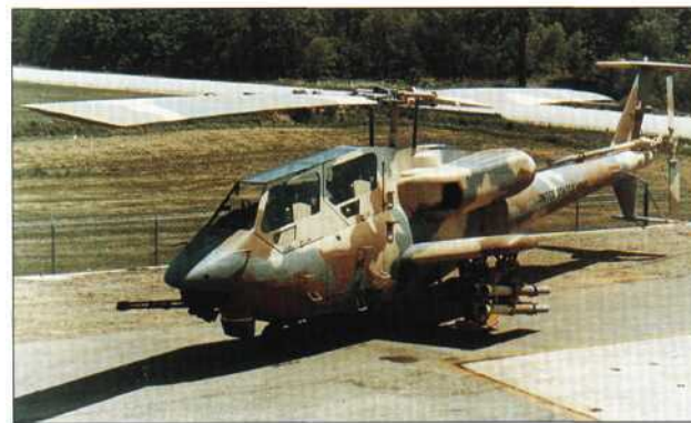
Right and below right: When the winners of the AAH initial evaluation were announced it was not surprising that Bell was selected as one of the two finalists. The wooden mock-up that Bell first produced was completely camouflaged; even the blades were painted. In contrast, the two prototypes wore an overall drab green scheme. Bell's YAH-63 design drew on all the company's experience with the AH-1 HueyCobra. It was beaten into the air by its Hughes rival, by a single day, in September 1975. The YAH-63 had an unhappy development and one of the two flying prototypes was lost in a crash. The other prototype, like the Cheyenne before it, survives today as an exhibit in the US Army Aviation Museum, at Ft Rucker, Alabama.
