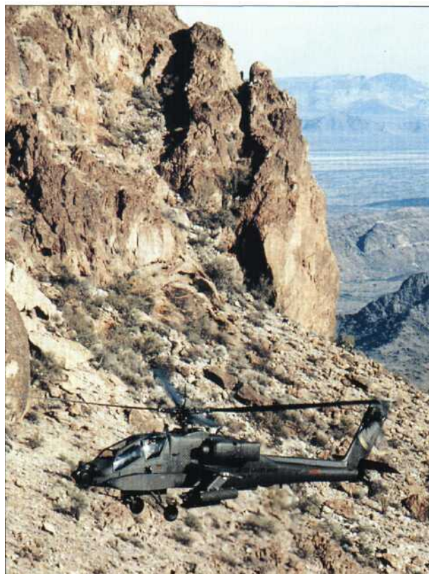
Above: Phase II testing revealed problems with the AH-64's rotor tips. As a result, the blade tips were swept back, leading to a reduction in compression loads and overall noise signature.
